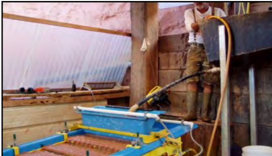
M7 table fed from overhead slurry tank
