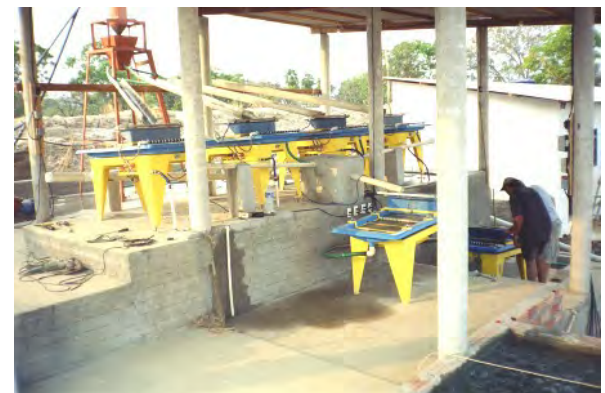
Alternate Production Configuration M7s in production series - final concentration on last M7 table
