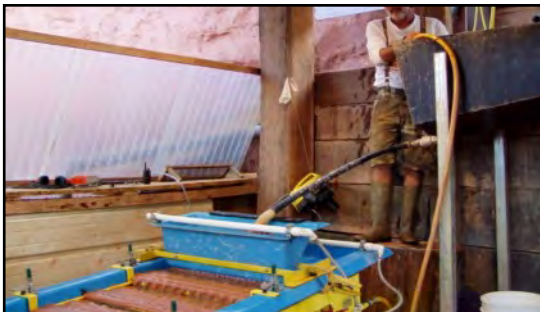
M7 table fed from overhead slurry tank
